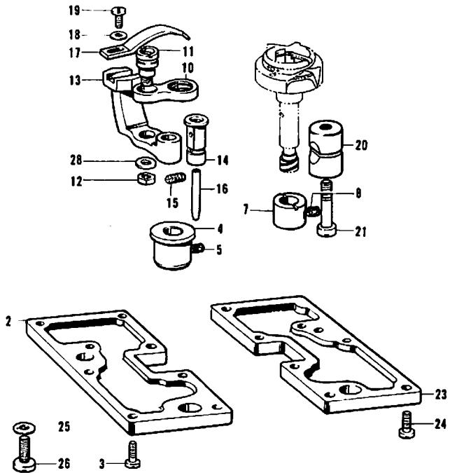
J. Rotary hook mechanism (2)[Standard]
