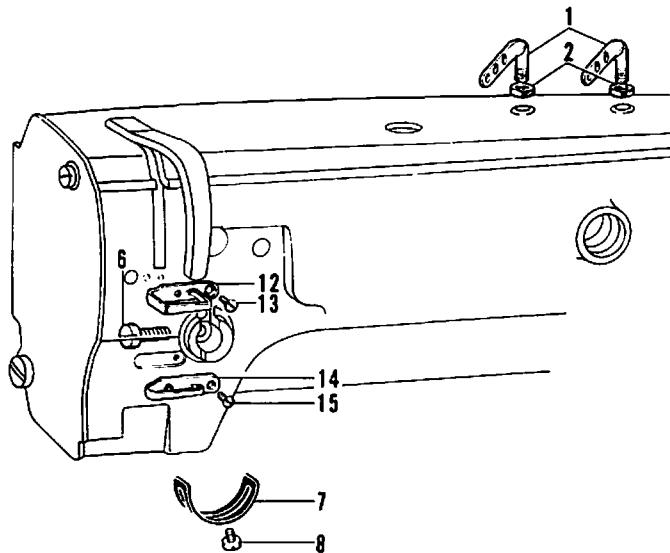
**B. Threading mechanism (2)(Standard)**
